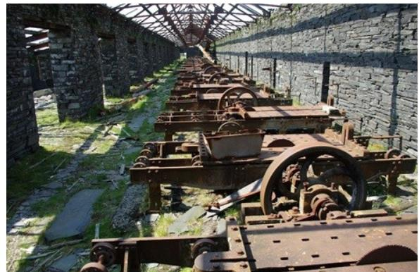
4: The inclines operated by gravity, with heavy loaded wagons descending and pulling up lighter empty wagons. The winding drums for the inclines can be seen.
