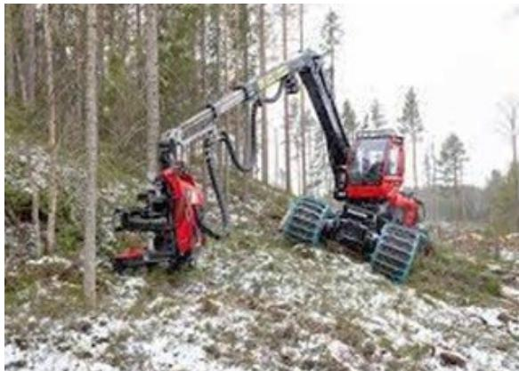
3: Other machines can pick up and transport the cut timber to a collection point. On very steep slopes, the machines are lowered by a cable from the top of the slope.
