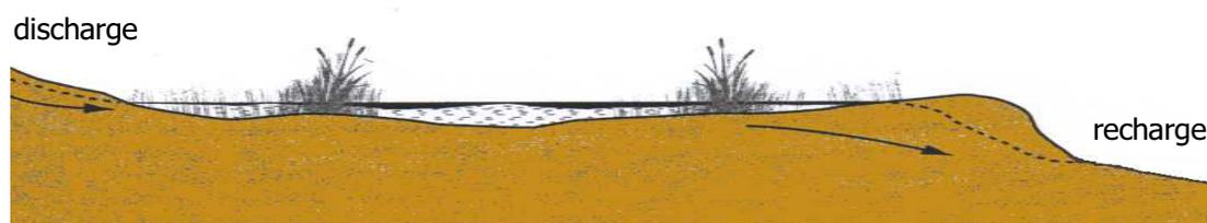
**Figure 3.184: Hillslope water flows within a blanket bog,** after Mitsch and Gosselink (2000)
