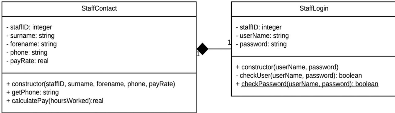
In the lower part of the box are listed the methods which can carry out actions involving **StaffContact** objects. The first is a **constructor** method, which creates new objects within the class and sets the values for the attributes. For example, if a new member of staff is appointed then a **StaffContact** object would be created containing their name, phone number and rate of pay.
