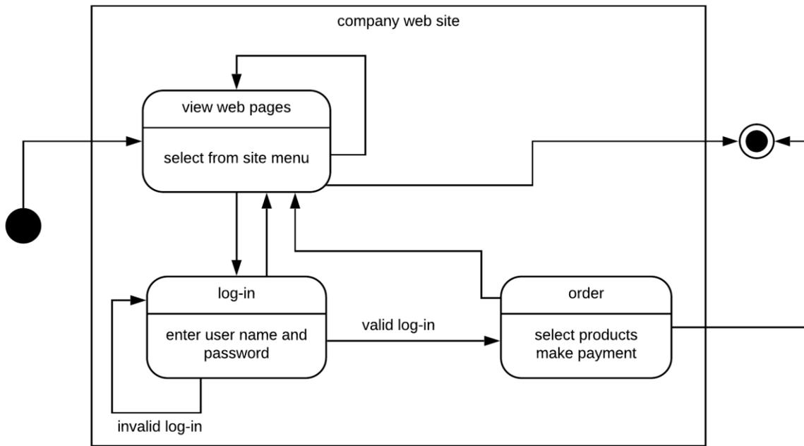
The computer system is outlined by a rectangle. The starting point for entering the web site is the black circle to the left of the diagram. Customers may then view the site, moving between pages by selecting from menu options. The upper section of the double box specifies the current situation or state, while the lower section indicates activities which may take place at this time.
