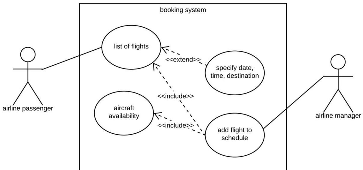
The airline manager will be responsible for adding flights to the schedule. Before a flight can be added, the manager must check that an aircraft is available. Since this is an essential operation, an arrow is drawn to the aircraft availability check and marked with the label `<<include>>`. Similarly, once a flight has been
