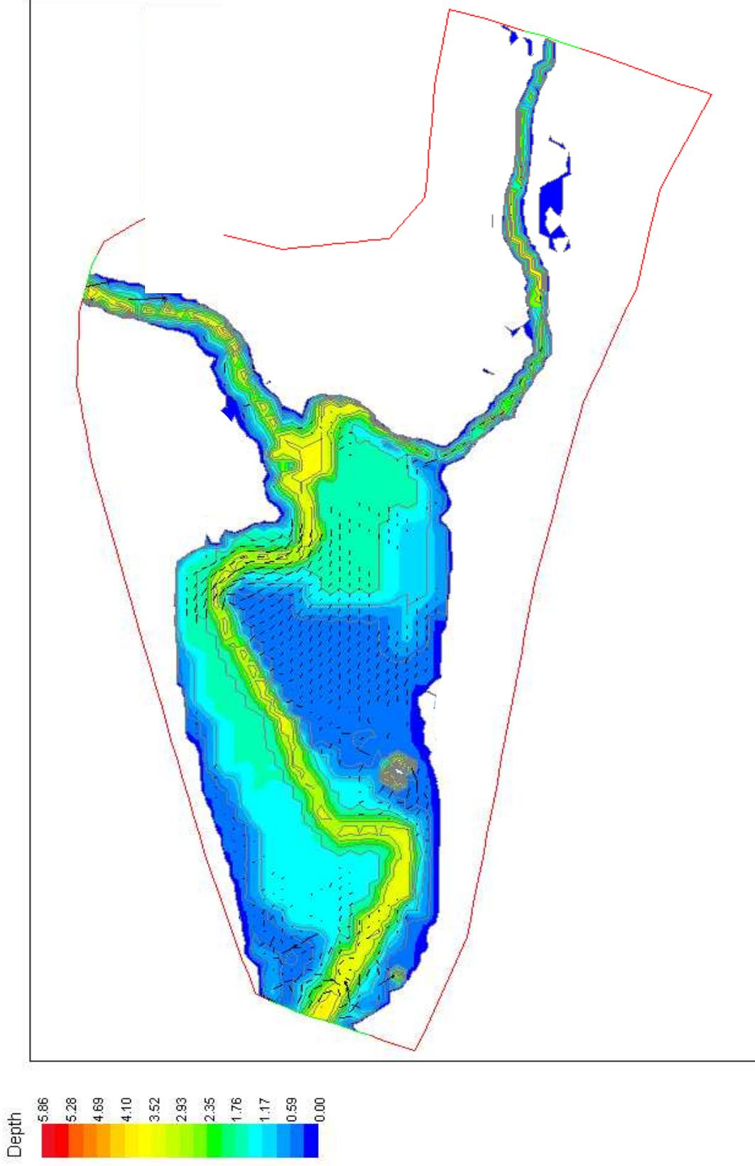
**Figure 3.254: Case 1. River flood with tidal inflow under current conditions**
