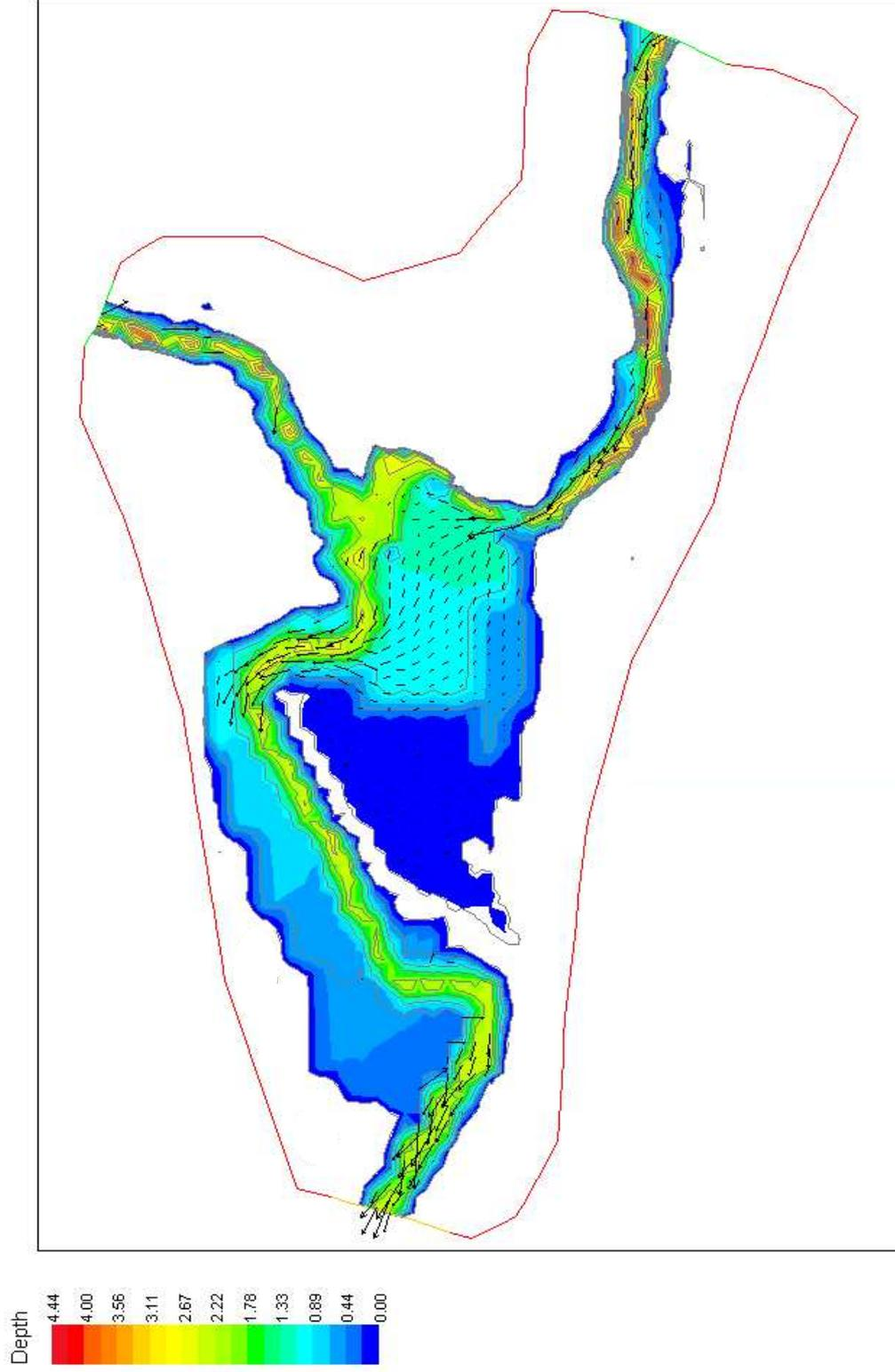
Figure 3.261: Case 3. River flood model after 0.5m gravel accumulation, falling tide
