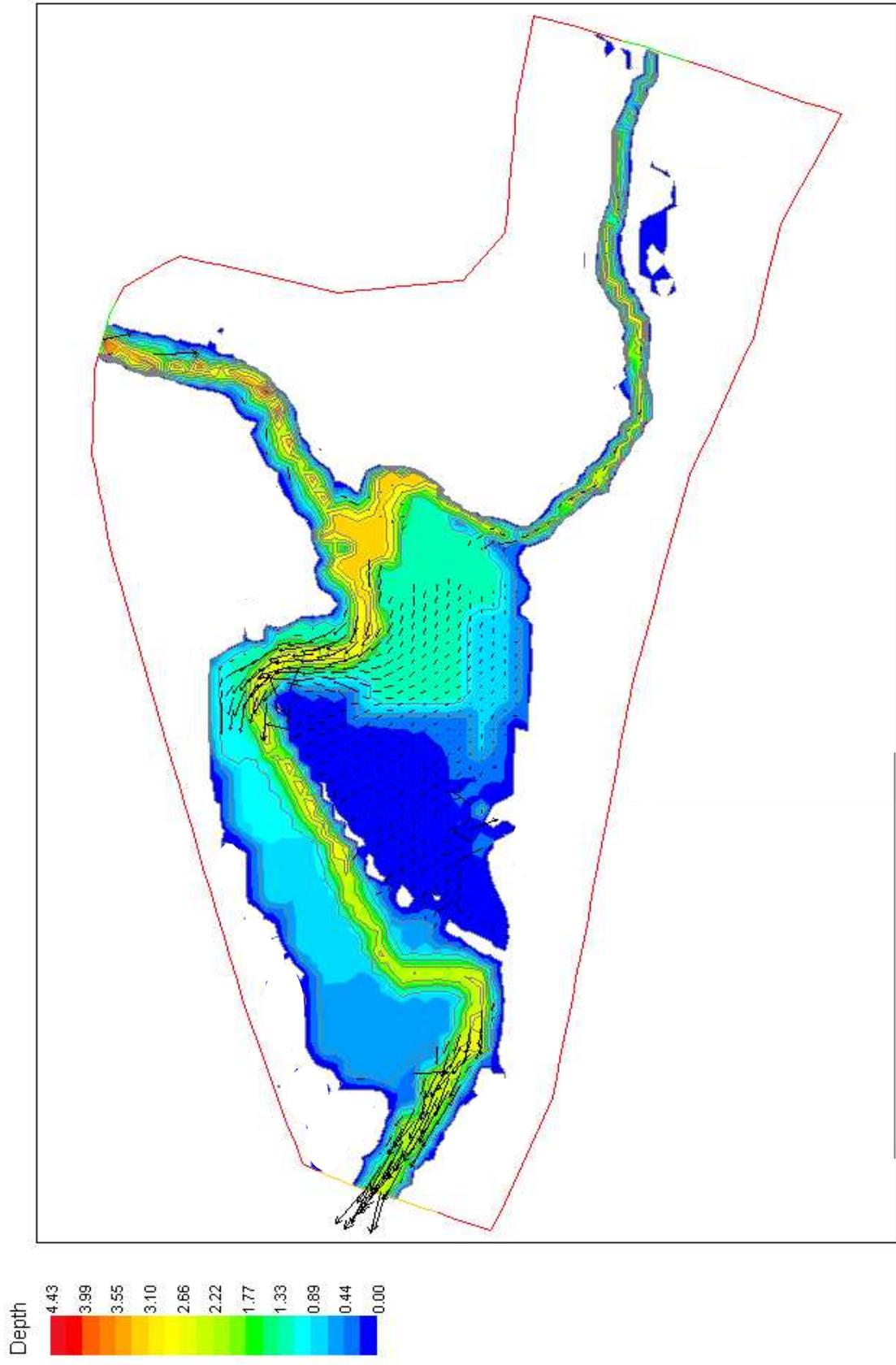
Figure 3.255: Case 1. River flood with tidal outflow under current conditions
