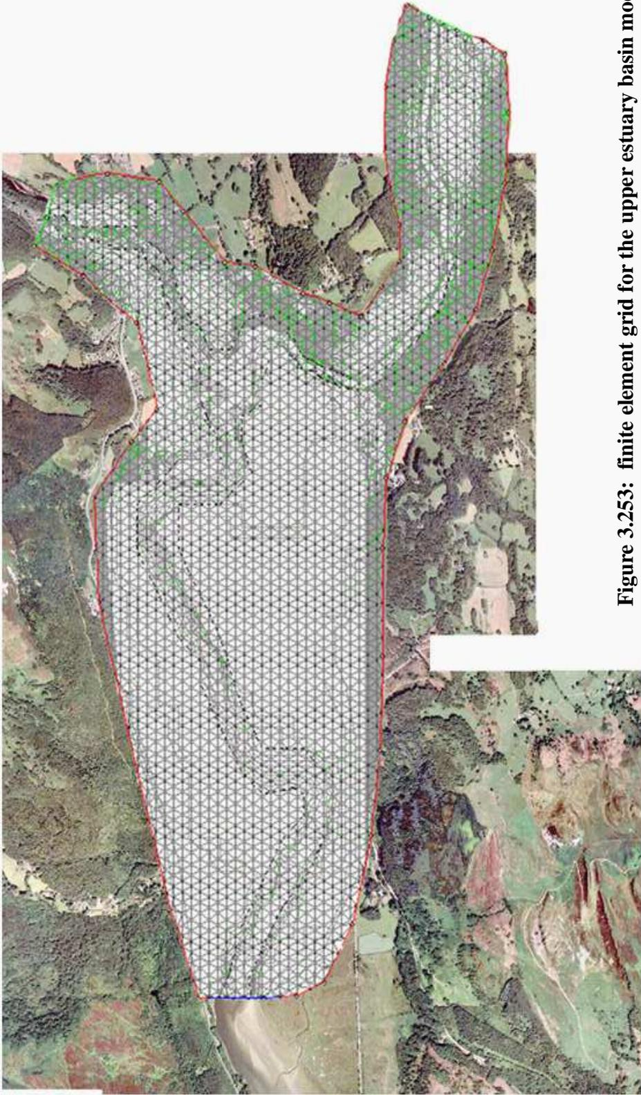
**Figure 3.253: finite element grid for the upper estuary basin model**
