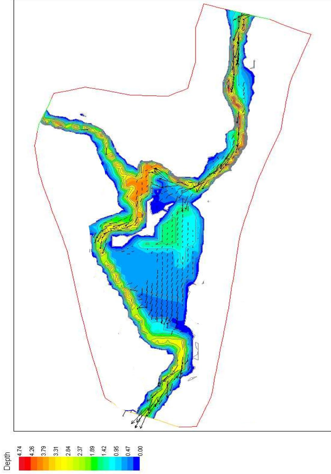
**Figure 3.258: Case 2. River flood event after land reclamation and construction of flood embankments at the head of the Mawddach estuary**
