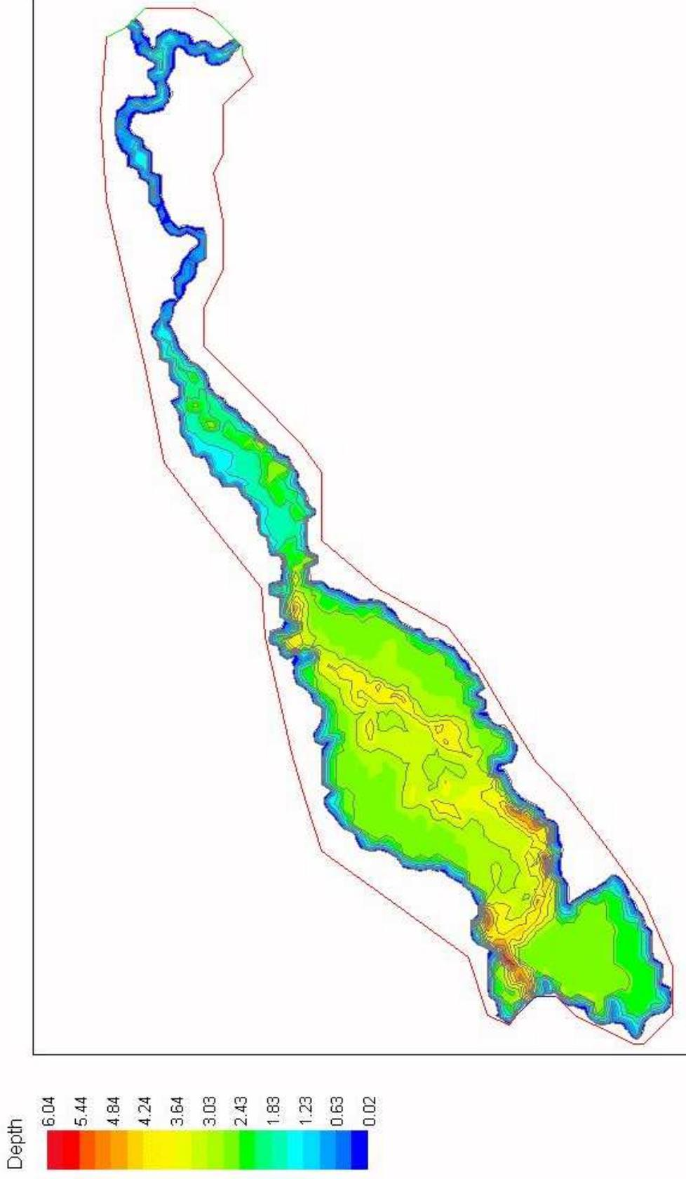
**Figure 3.245a: Simulation of a 4m tide maximum water level for the Mawddach estuary.**
