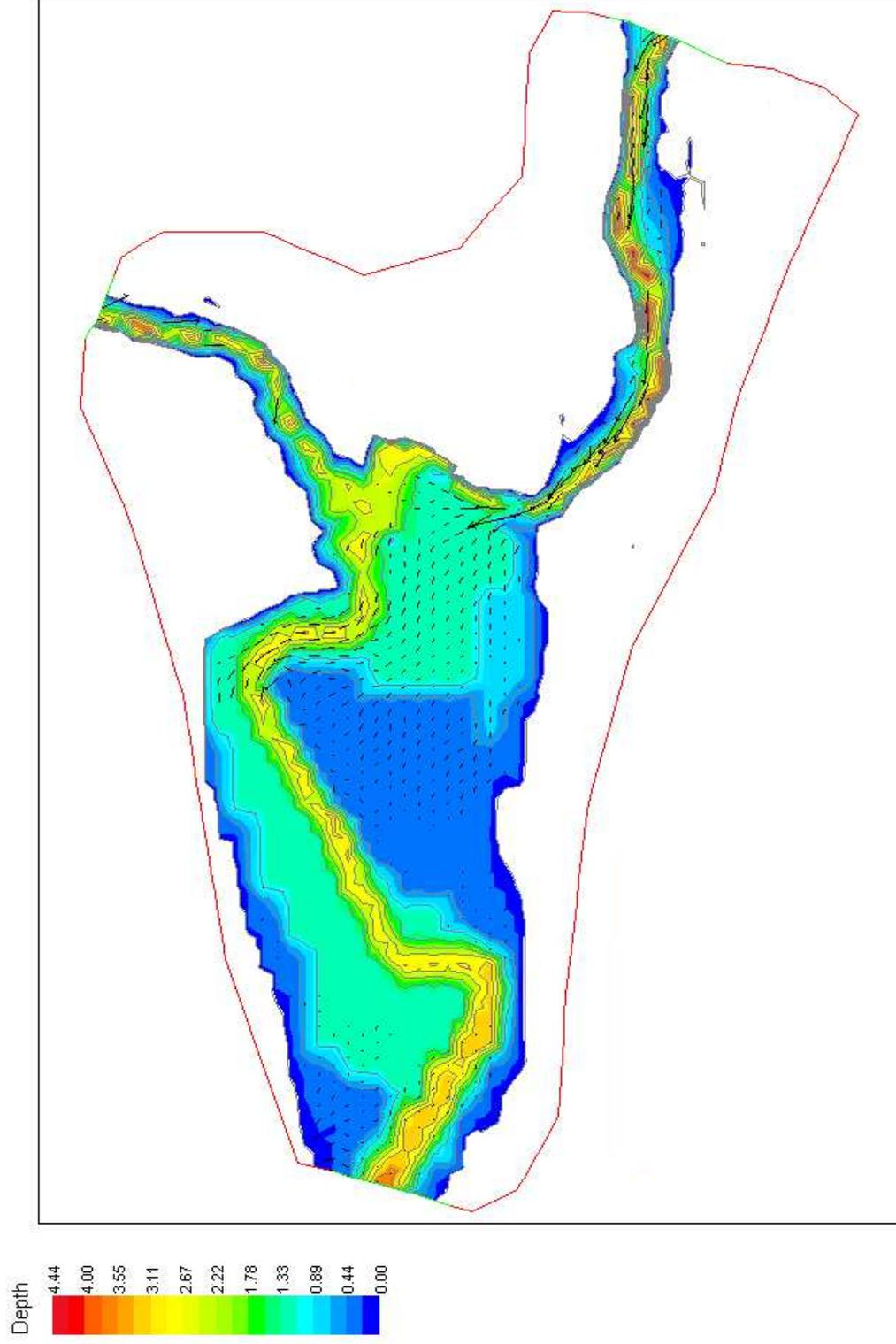
**Figure 3.260: Case 3. River flood model after 0.5m gravel accumulation, rising tide**
