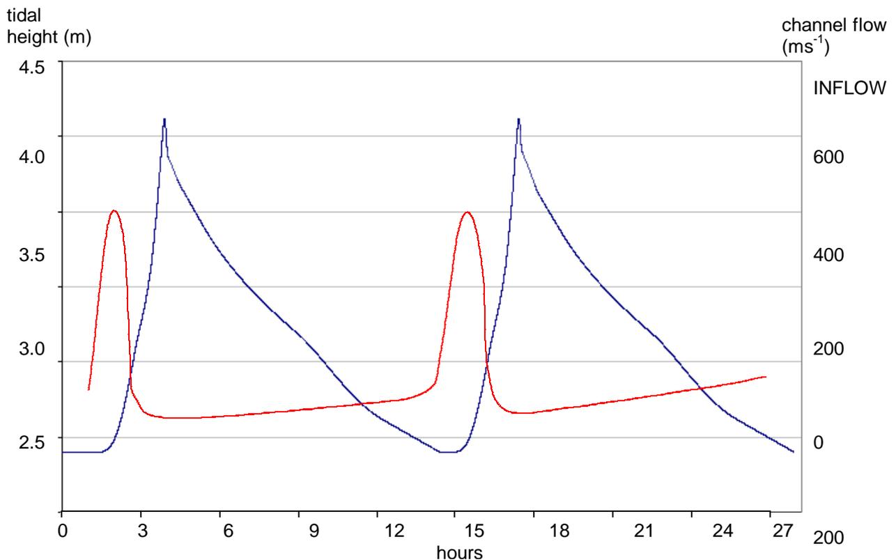
**Figure 3.252: Simulated water height (blue) and channel flow (red) at Penmaenpool bridge during tidal flood-ebb cycles**
