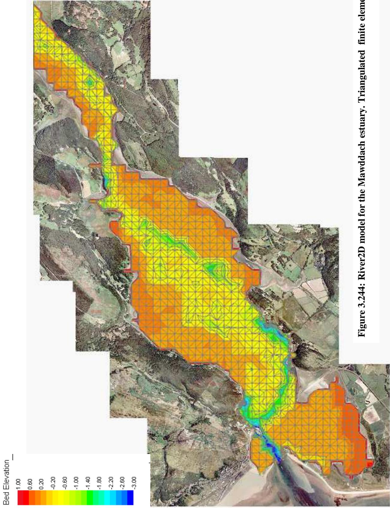
**Figure 3.244: River2D model for the Mawddach estuary. Triangulated finite element grid**
