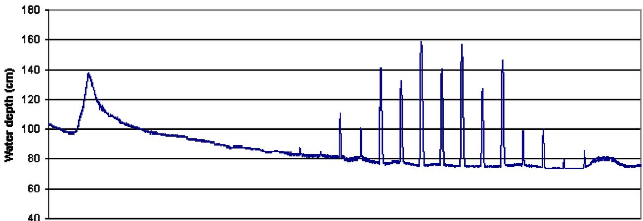
**Figure 3.241: Hydrographs for recording points at the mouth and head of the Mawddach estuary, 10-24 February 2003**
