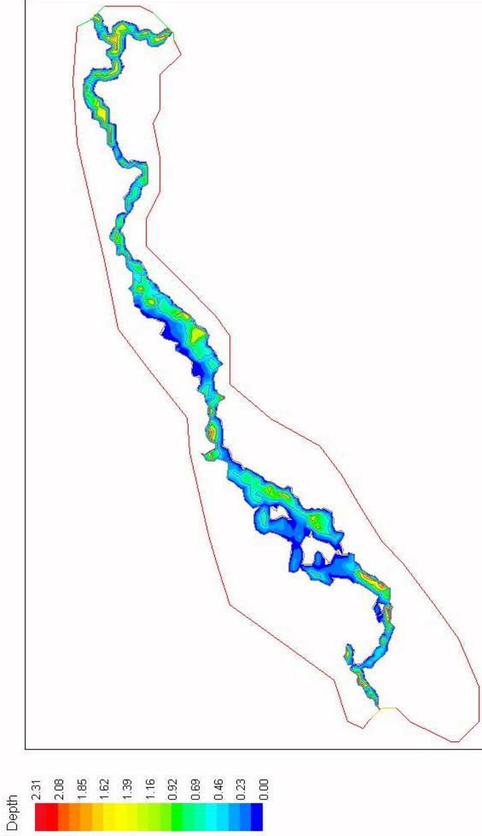
**Figure 3.245b: Simulation of a 4m tide minimum water level for the Mawddach estuary.**
