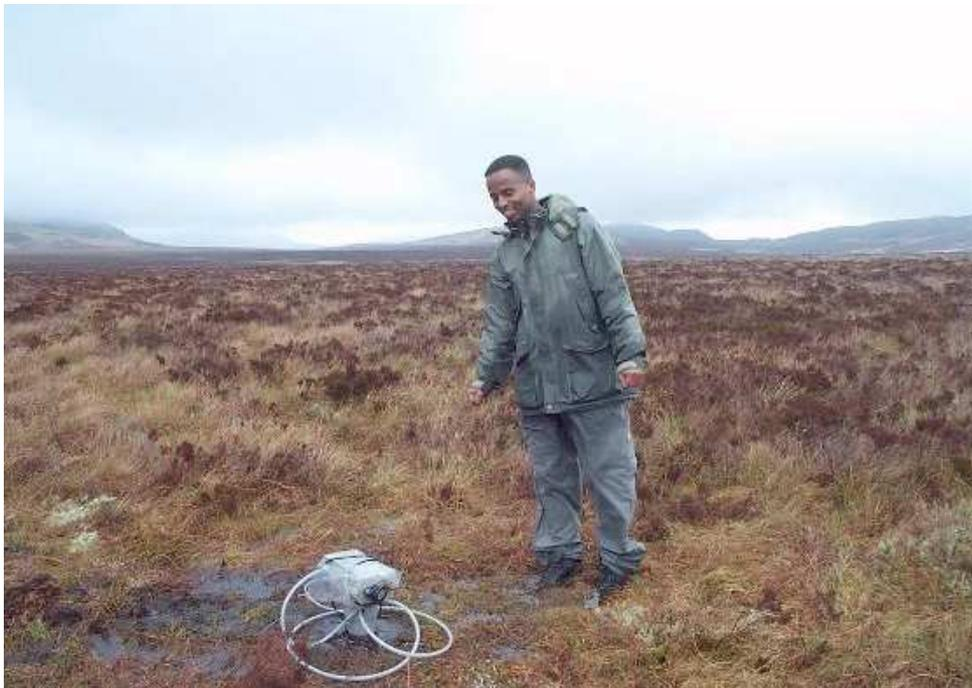
**Figure 3.203: Waen y Griafolen borehole with water depth recorder**
