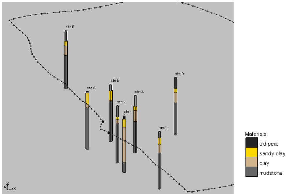
**Figure 3.209: Stratigraphic sequences plotted on the MODFLOW model from geophysical data**
