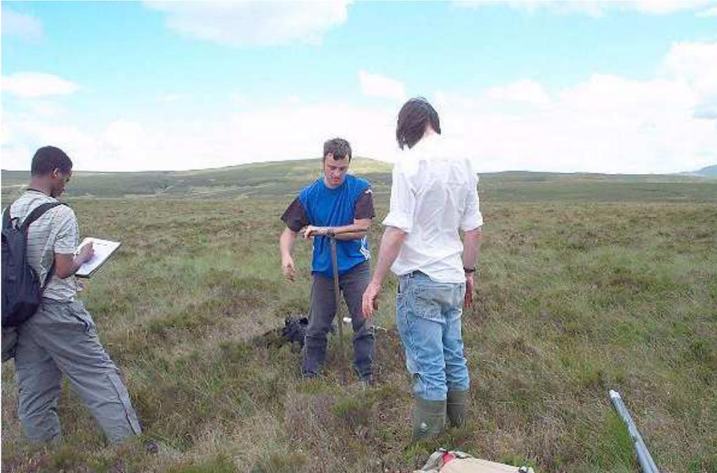
**Figure 3.205: Emplacing a dip well tube in older peat at site 7, Waen y Griafolen**
