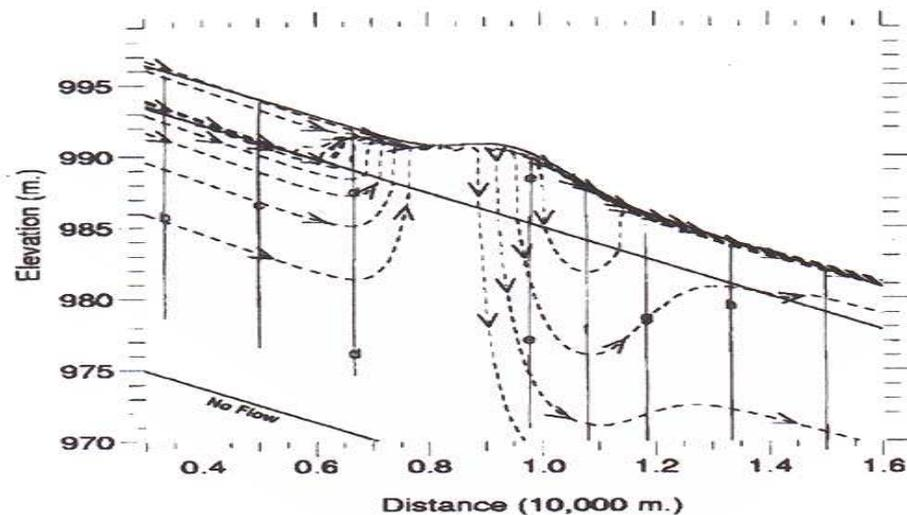
**Figure 3.186: Model showing water flow pathways around a spring seepage area associated with a localised peat dome, after Reeve, Siegel and Glaser (2000).**
