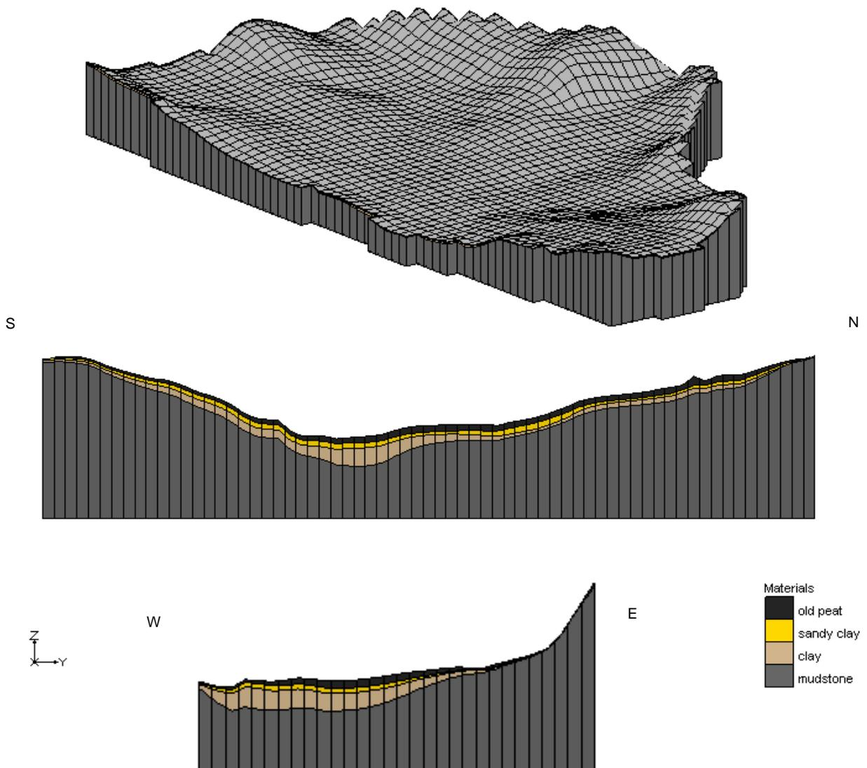
**Figure 3.210: Waen y Griafolen MODFLOW three-dimensional grid, showing example South-North and West-East cross sections.**
