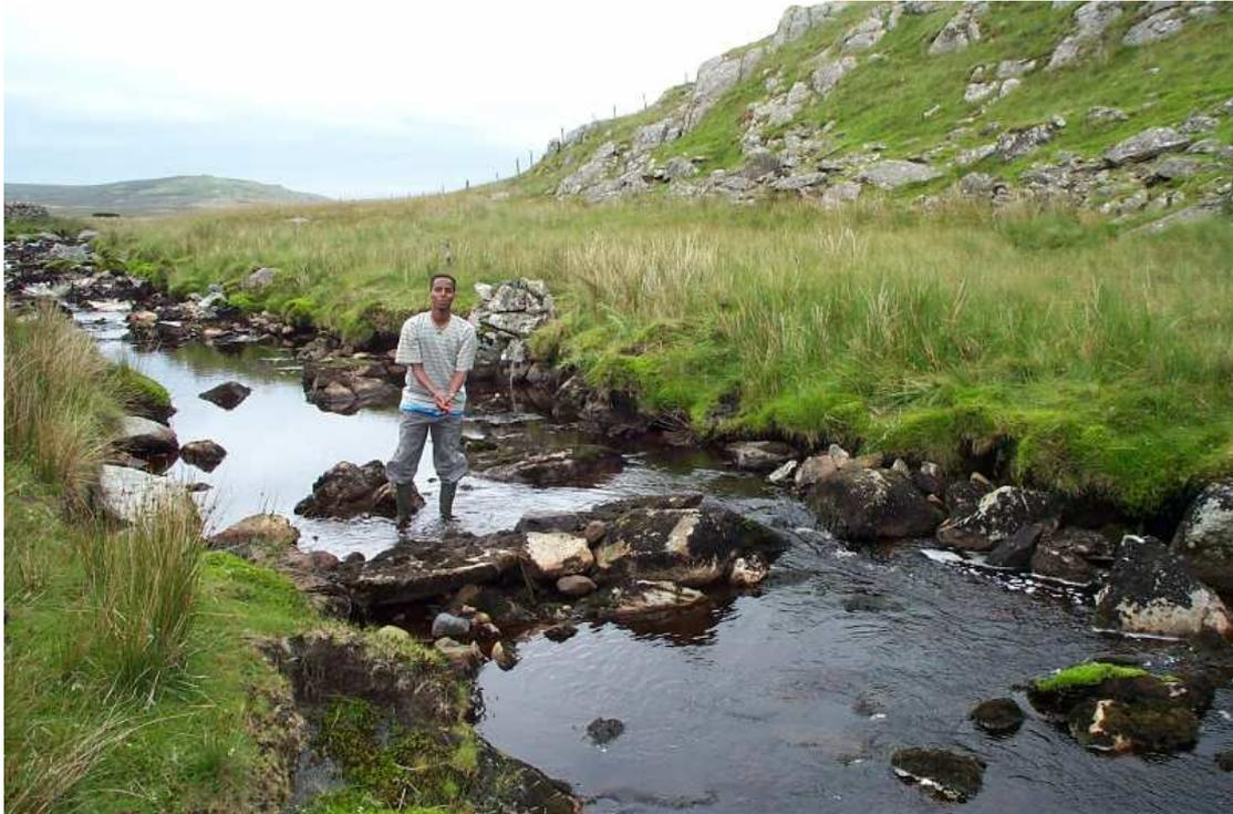
**Figure 3.207: Outlet stream hydrograph site, Waen y Griafolen. A barometric depth recorder is situated in the pool upstream of the V-notch weir.**
