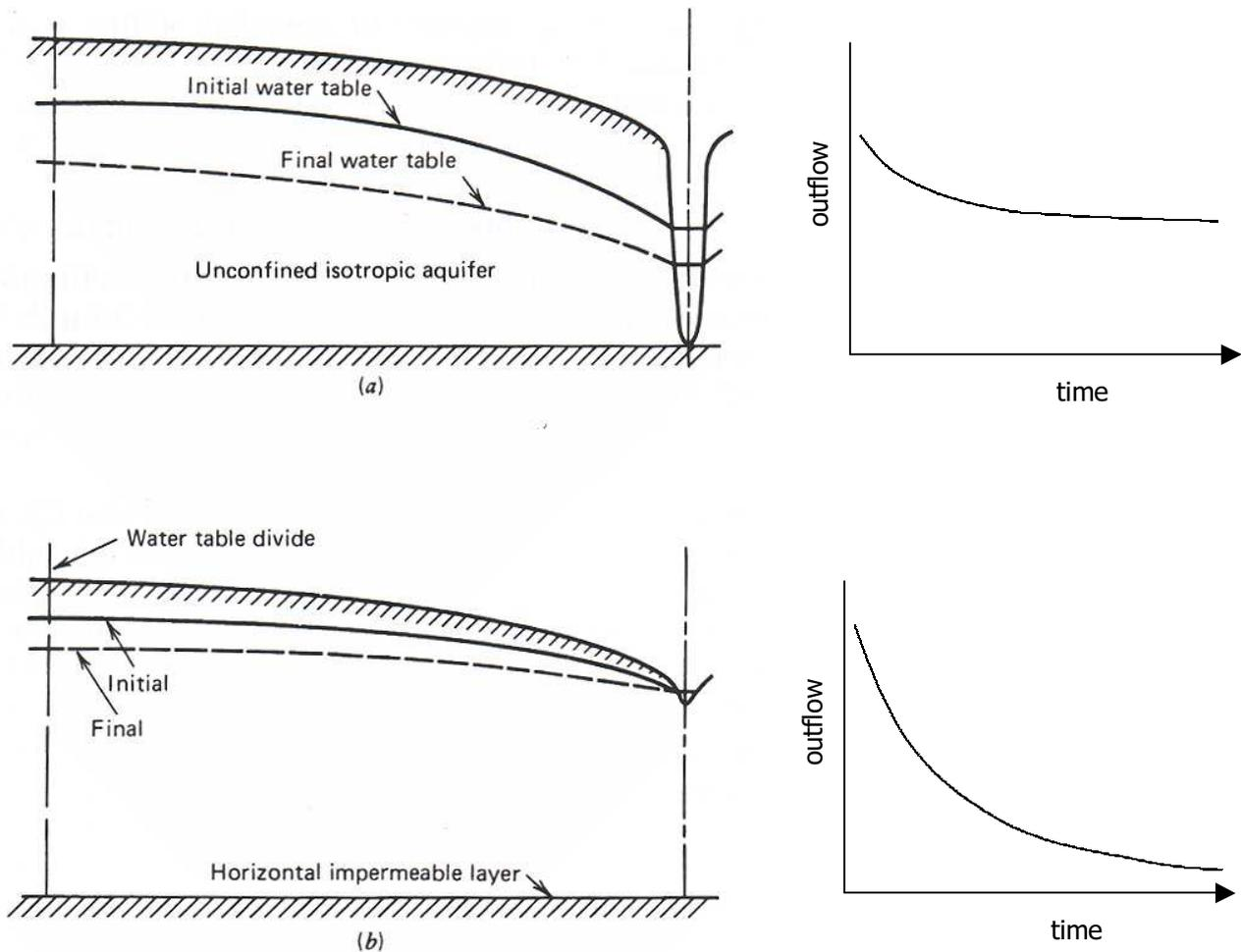
**Figure 3.187: Models for stream penetration depth and outflow hydrograph patterns.**
