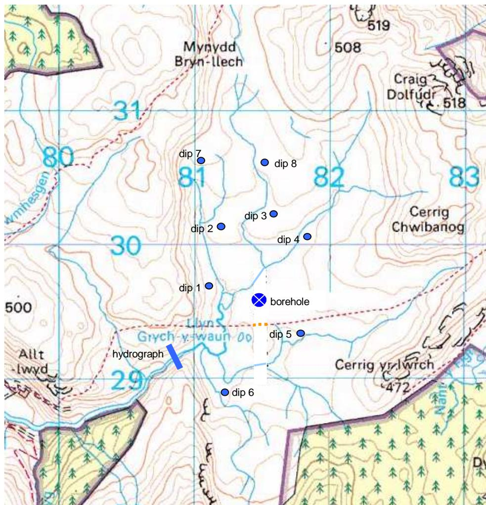
**Figure 3.206: Locations of dip wells, borehole water depth recorder and hydrograph site, Waen y Griafolen**
