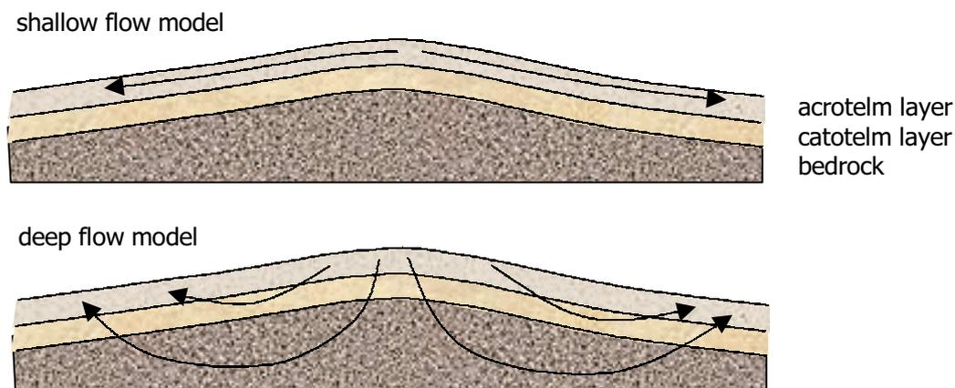
**Figure 3.185: Models for water flow within a blanket bog,** after Reeve, Siegel and Glaser (2000)
