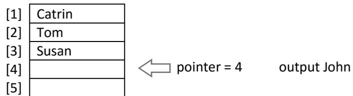
The process can continue, with the output of each data item and the pointer moving upwards until the array is again empty. The **first data item input** will be the last **data item output** from the array.
