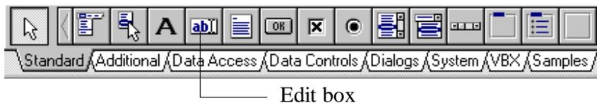
Place two **edit boxes** on the form. Select the **Label** component and place the labels 'A' and 'B' alongside the edit boxes:
